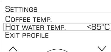
The different setting options can be selected with the selection buttons **^** and **v** **4**.
