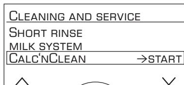
The **start** button **8** flashes while the different Calc'nClean processes are running. The figures on the top right indicate the progress of the programme.
